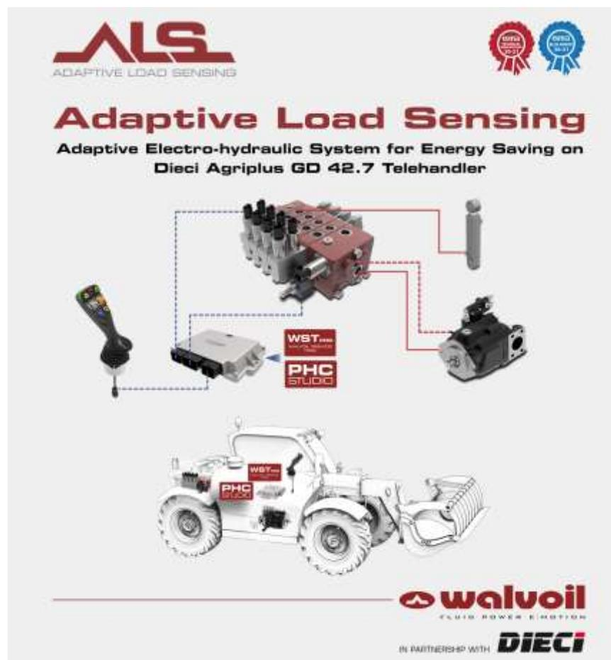
ALS is made of a directional control valve, an electronic joystick, and an electronic control unit, with customizable modular software developed by Walvoil. The control unit collects information from the operations on the controls and from the machine sensors, and acts on the Load Sensing device, adapting the hydraulic pressure differential to the maximum efficiency value required by the vehicle.
